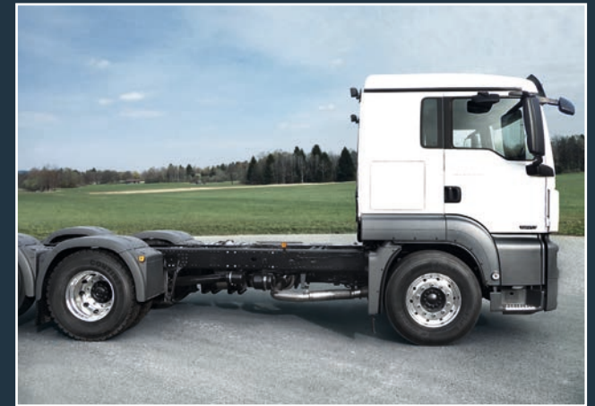
Right side of frame free for side loader mounting
