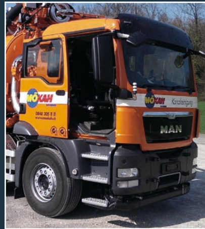
Cab with sliding door (can be moved left and right)
