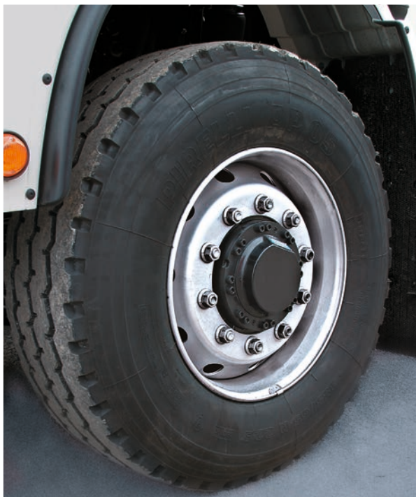
Front axle with hydrostatic wheel hub motors
