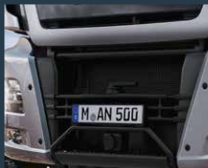
Steel bumper with centred towing eye and hinged front step. Particularly robust protective grill in front of radiator.
