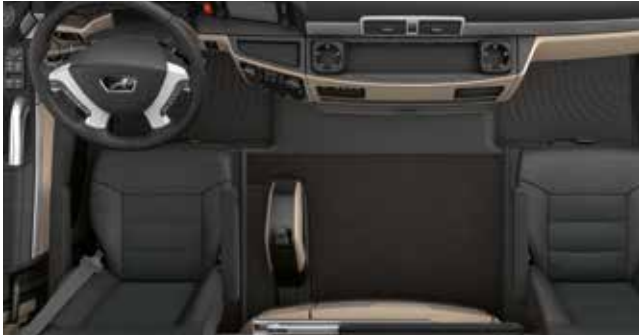
Rearranging the TipMatic switch and parking brake creates additional space
