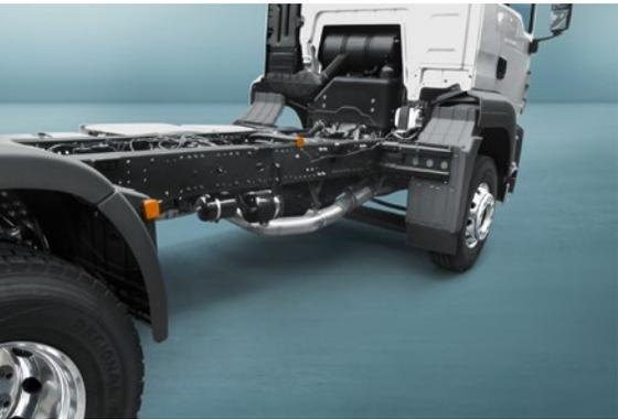
Clearance on the right with relocated exhaust silencer
