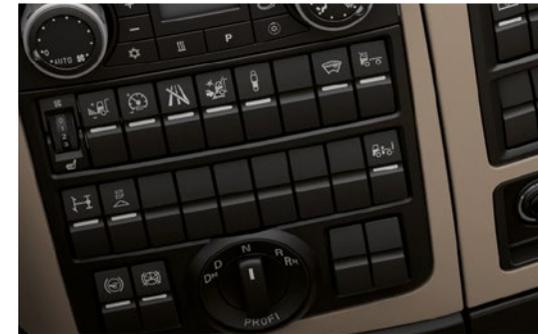
Rotary switch for MAN TipMatic®.
