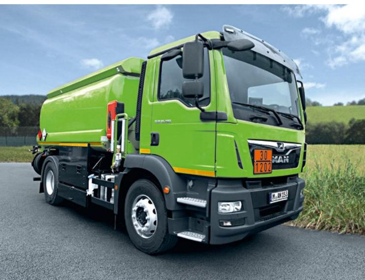
A robust model is the MAN TGM with a powerful six-cylinder engine of up to 251 kW (340 hp) – perfect for solo and light trailer operation. Optionally available with steered, liftable trailing axle. It results in a longer technical wheelbase which increases the front-axle load and optimises the good steering qualities of the vehicle, whatever the load.
