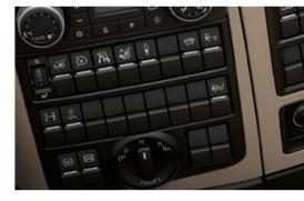
Rotary switch for MAN TipMatic®.
