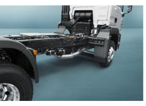
Clearance on the right with relocated exhaust silencer
