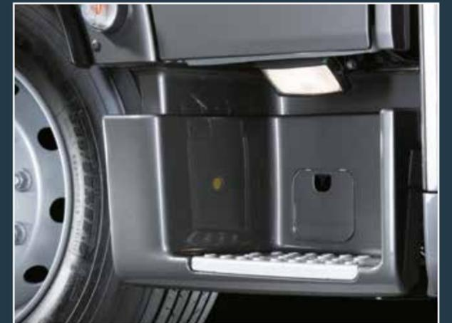
Manoeuvring light at the co-driver's step unit
