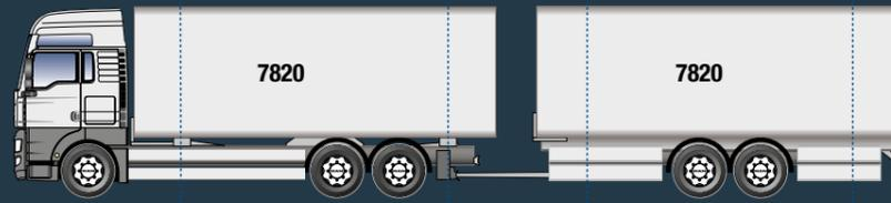
Wheelbase/overhang: 5100 + 1350/1850 mm for permanent operation with trailer
