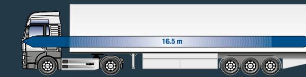
Overall length of semitrailer tractor + semitrailer
