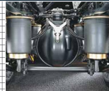
Air suspension with ample raising and lowering travel of 240 mm.
