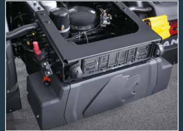
Compressed-air tank at the rear of the frame
