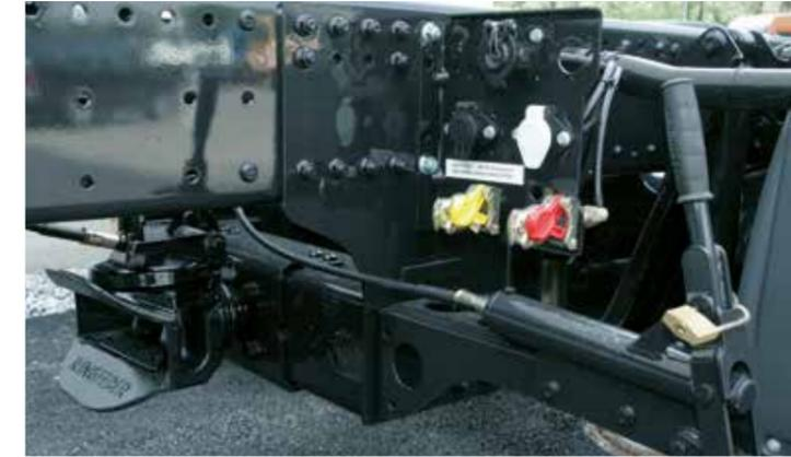
Low coupling mount with trailer coupling. Return 1400 mm (standard) or 1600 mm (volume). Brake and electrical connections to customer specification on driver's or co-driver's side, behind trailing axle.
