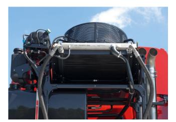
Additional radiator for engine + torque converter clutch
