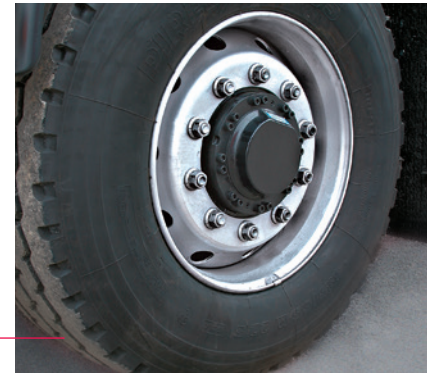
Front axle with hydrostatic wheel hub motors.
